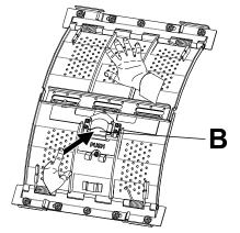
You can also push with your finger on B. We suggest you to use gloves. Load the linen in the inner drum. Be careful to distribute it correctly.
