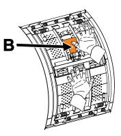
Close the inner drum doors and press them to check the good working of the mechanical safety device (B).
