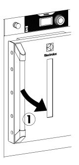
Open the unloading door with the handle (1).
