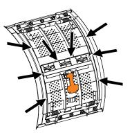
Check that no piece of linen is wedged between the doors and the inner drum.
